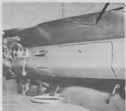
Arrow shows how sun rays reflected by mirror burned polyvinyl-covered dashboard.
